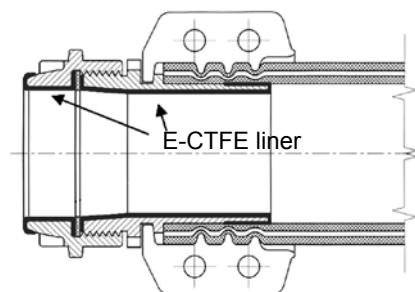
E-CTFE coated couplings resist the most aggressive chemicals, even so corrosive that the couplings made of AISI 316 acid resistant steel fail. When corrosion is the case, it is recommended to use either expensive couplings made of special nickel-based alloys (e.g. Hastelloy) or (not so expensive) AISI 316 steel couplings with powder coated E-CTFE liner.
