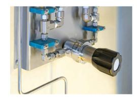
Precision metering valves for general purpose application, also suitable for panel mounting. 3 valve versions are available depending on required working pressure, flow rate and accuracy. Can be supplied as straight or angle valve. Several handle options, also a Vernier handle to facilitate easier valve opening control. This range of valves includes a unique, patent version with an integrated ball valve to allow both full flow control and complete shut-off at the same time.
