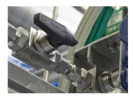
UCV — Ultra Clean Valves, special type of diaphragm valves designed for high purity applications, for example in the semiconductor industry. Available as manual valves or with a pneumatic actuator.
