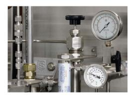
Precision needle valves, depending on their construction, are used as shut-off valves to control the flow and for dosing media. There are 4 types of stems:
