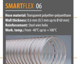
Characteristics: Lightweight, flexible hose designed for the extraction of dust and small particles. Used in the woodworking and furniture industries. Highly resistant to abrasion and mineral oils, flexible at low temperatures, even below zero. According to BGI 739, the hose is considered electrically conductive after grounding the wire helix. The hose is marked with an arrow indicating the correct flow direction. Other diameters available in the range of
