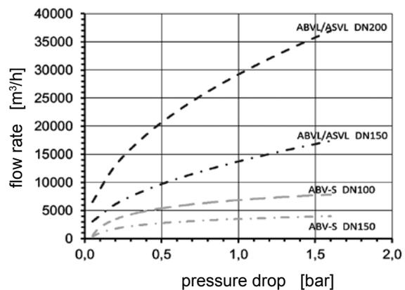
Test parameters: medium water, temperature +20°C.
