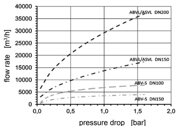
Test parameters: medium water, temperature +20°C.
