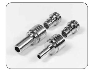
Material:Chrome-plated brassWorking press.:Up to 25 barWorking temp.:Up to +150°CSealing:Viton
