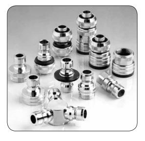
Material:Chromium plated brassWorking press.:Up to 25 barWorking temp.:Up to +80°CSealing:NBR - cannot be used with fuel and oil<br/>(option - Viton).<br/>For valve O-ring made of EPDM.
