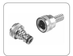
Material:Chrome-plated brass (matt - satin)Working press.:Up to 25 barWorking temp.:Up to +150°CSealing:NBR - not suitable for oil and petrol (Viton seal as an option). EPDM O-ring for a valve.
