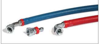
Note: PUSH-ON hoses can also be assembled using clamps or ferrules, provided that the clamp and tail of the fitting do not damage the relatively thin wall of the hose, so never use PUSH-ON fittings with large and sharp serrations.
