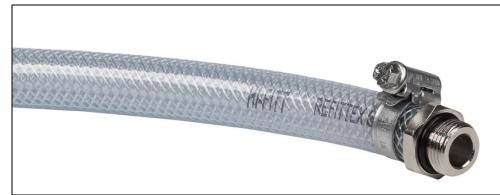
REFITTEX CR hose assembled with nickel-plated brass ferrule with 3/8" BSP male thread (MW-2119008), by means of a hose worm drive clamp. The fitting enable easy connection with other pneumatics components without a need for additional seals.
