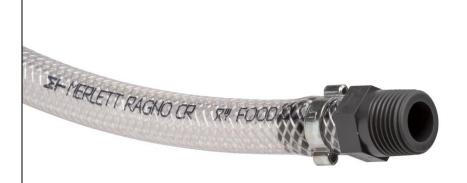
RAGNO CR DN12 hose assembled with a plastic (polyamide) ferrule with BSPT male thread (NA-7100013012), by means of the EAR CLIP. Incidentally, the name -RAGNO means spider in Italian, which may refer to the intricate web of the braid that provides this hose with the pressure resistance.
