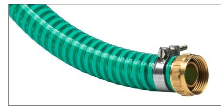
LUISIANA SE DN20 hose assembled with a brass fitting with a 3/4" BSP female thread (NT-27250A4) clamped with a MINI screw clamp, designed for water with plant protection products in botanical garden in Ukraine. Practically smooth external layer of the LUISIANA SE DN20 hose and its rather soft wall facilitates proper and tight clamping to the ferrule even with a light hose MINI clamp.
