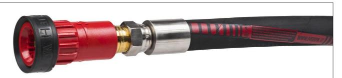
CHICAGO hose DN19 with 3/4" BSP female thread hydraulic fitting, with flat seal, in AISI 316 stainless steel, crimped with TI-L-33-12-SS ferrule, with HANDIFIGHTER 20 bar jet nozzle. Working pressure of a hose assembly with a jet nozzle is 20 bar. To take full advantage of the capabilities of the hose, 40 bar jet nozzle should be attached.
