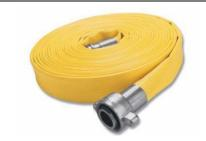
DN 20 hose and DN 25 hose in 20 m length, with 42 mm claw couplings or with screw-connection DIN 8537/20033 couplings at both ends are often used for compressed air in the construction industry, for jack hammers and augers drills.
