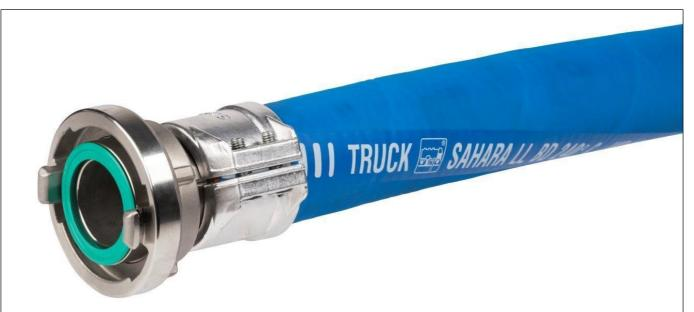
SAHARA LL BD hose DN51 with STORZ coupling (ST-13-066050-43) in stainless steel mounted with an aluminium safety clamp. Fitting (type ST-13...) has a smooth tail and a safety lock matching a safety clamp. STORZ gasket is made of Viton, heat resistant, standard for STORZ stainless steel couplings. On road tankers for bulk materials, a cheaper STORZ coupling made of aluminium is often used. It has a heat resistant silicone gasket.
