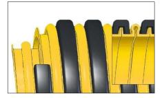
The hose and cuffs are also sold separately, then the cuffs can be screwed onto the hose and glued with a special adhesive. Short hose sections (e.g. 1 m long) with cuffs can be used as a protection hose placed on the edge of a sewer opening into which a high pressure cleaning hose or inspection camera cable is inserted. The protection hose is kept in position by a rope attached to the cuff with a clamp.
