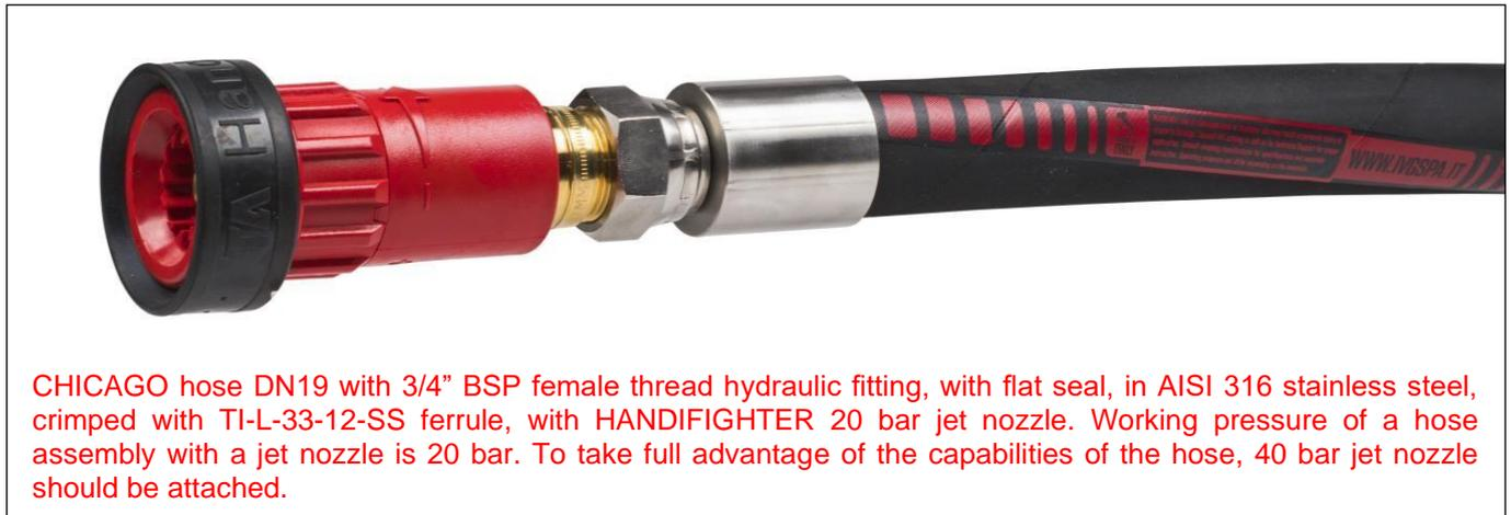
CHICAGO hose DN19 with 3/4" BSP female thread hydraulic fitting, with flat seal, in AISI 316 stainless steel, crimped with TI-L-33-12-SS ferrule, with HANDIFIGHTER 20 bar jet nozzle. Working pressure of a hose assembly with a jet nozzle is 20 bar. To take full advantage of the capabilities of the hose, 40 bar jet nozzle should be attached.
