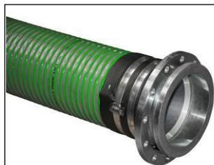
A massive ARIZONA SE hose DN250 L= 6 m to be used on a pump suctioning dirty water and sludge. The hose with swivel flange connectors DN250 PN10 in zinc-plated carbon steel attached using a band clamping system. A sleeve under the bands levels the hose surface to ensure even compression and prevent the band from cutting in.
