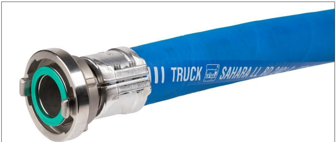
SAHARA LL BD hose DN51 with STORZ coupling (ST-13-066050-43) in stainless steel mounted with an aluminium safety clamp. Fitting (type ST-13...) has a smooth tail and a safety lock matching a safety clamp. STORZ gasket is made of Viton, heat resistant, standard for STORZ stainless steel couplings. On road tankers for bulk materials, a cheaper STORZ coupling made of aluminium is often used. It has a heat resistant silicone gasket.
