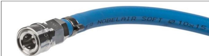
SUPER NOBELAIR SOFT hose DN10 with NITTO KOHKI quick release coupling socket (NK-30SH-SS) in stainless steel mounted with a stainless steel EAR CLIP-W with inner insert. The ear clip with the inner insert grips the hose tight and protects its cover.
