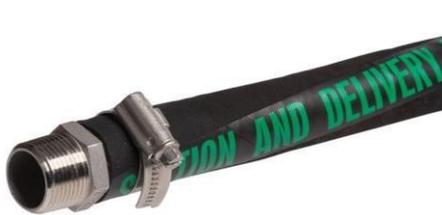
TORONTO LIGHT hose DN19 with AISI 316 stainless steel fitting 3/4" BSPT taper male thread (NM- VT123-12), worm drive clamp in AISI 316 steel (AB-03017500).
