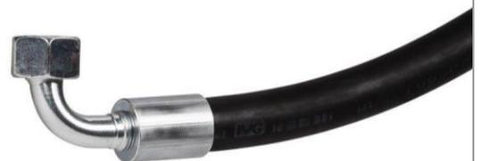
AIR20 hose DN6 with RECTUS quick release coupling socket for pressure-free disconnection (RE-26KETF06MPN), mounted with EAR CLIP in zinc-plated steel.
