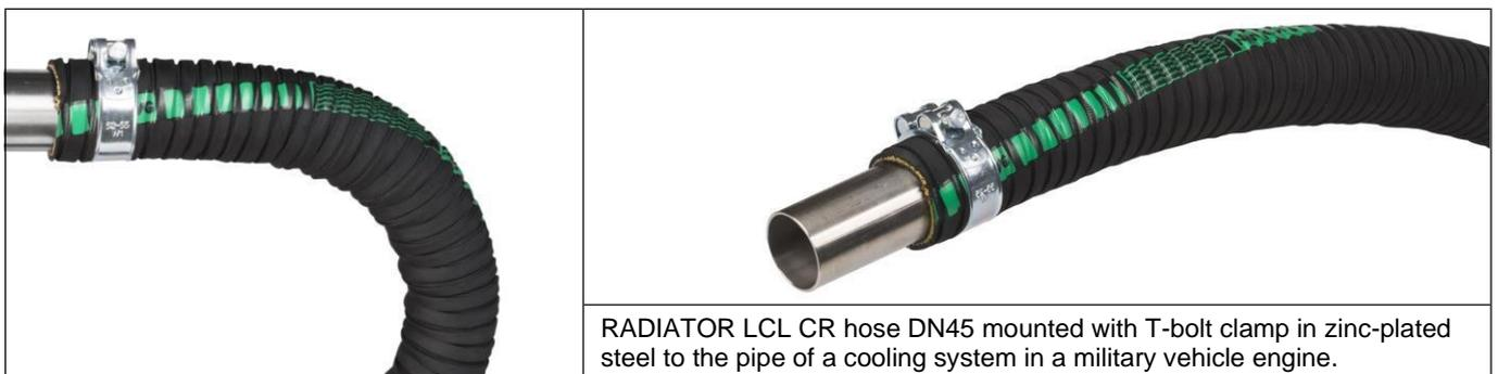
RADIATOR LCL CR hose DN45 mounted with T-bolt clamp in zinc-plated steel to the pipe of a cooling system in a military vehicle engine.
