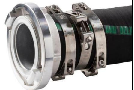
TORONTO LIGHT hose DN110 with aluminium STORZ coupling (lug distance 133 mm, ST-12-133110-11), W5 version DPC double bolt clamp in AISI 316 steel; 3 clamps placed between the serrations of the fitting.
