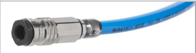
NOBELAIR AS/R hose DN6 with TEMA chrome-nickel-plated brass quick release coupling socket (TA-P-1400) mounted to the hose with special 1/4" BSP male thread fitting with a screw-on sleeve that is screwed with the socket and sealed via a flat gasket.
