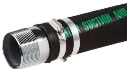
TORONTO LIGHT hose DN51 with KING NIPPLE fitting 2" BSPT male thread (AC-CNP-200) in zinc-plated steel, W1 version worm drive clamps (AB-03009006) also in zinc-plated steel.
