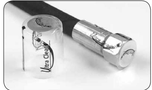
Clean seal capsules leave absolutely no particles or sticky surface. They perfectly protect the hose assemblies or pipes from contamination until they are removed. Removal includes gripping the black pull tab, then ripping the pull tab upwards and finally slipping the clean seal capsule off the hose assembly or pipe. Clean seal capsules are single use and cannot be used again.
