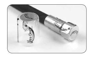
Clean seal capsules leave absolutely no particles or sticky surface. They perfectly protect the hose assemblies or pipes from contamination until they are removed. Removal includes griping the black pull tab, then ripping the pull tab upwards and finally slipping the clean seal capsule off the hose assembly or pipe. Clean seal capsules are single use and cannot be used again.
