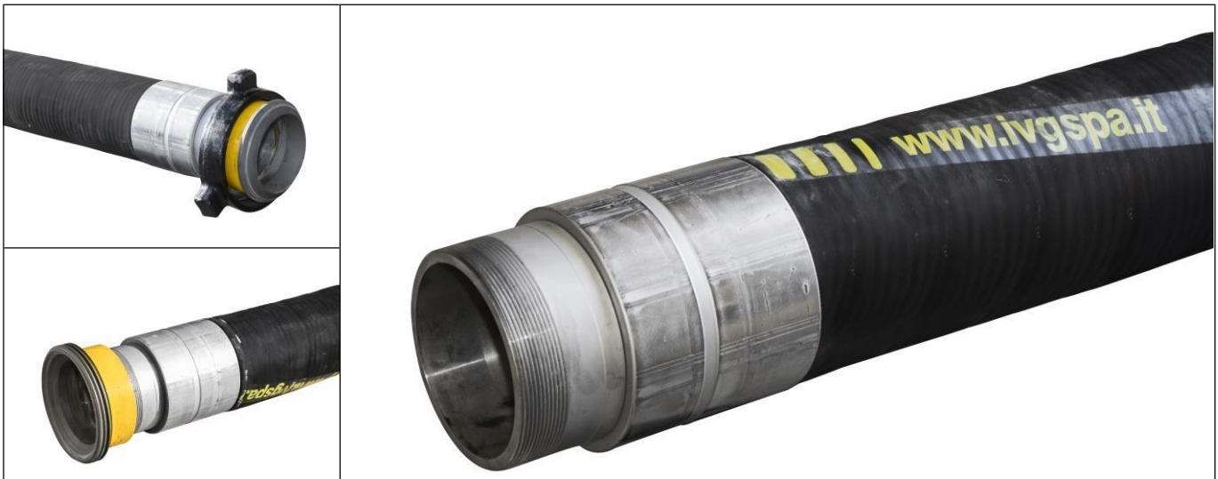
FUEL HARDWALL hose DN152, length 8 m, with carbon steel NPT 6" male tapered thread fittings at both ends. The fittings crimped with carbon steel ferrules - external crimping. HAMMER LUG union 6" Fig. 100 male part with a female thread nut is mounted at one end of the hose, and HAMMER LUG union 6" Fig. 100 female part at the other end. The complete hose assembly will be used for drilling mud in a land-based application.
