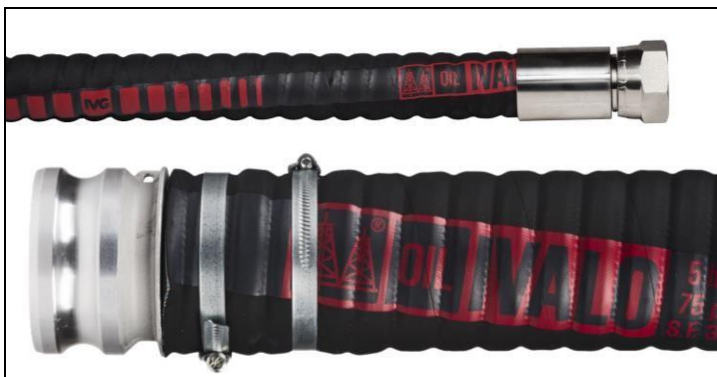
IVALO hose DN25 with 1" BSP female thread fitting in AISI 316 stainless steel (TI-ZBW110-16-16-SS) assembled with a ferrule (TI-L-37-16-SS) in AISI 304 stainless steel and IVALO hose DN76 with aluminium CAMLOCK E 3" coupling (AC-E-300-A) assembled with clamps (AB-03009009) in zinc-plated steel.
