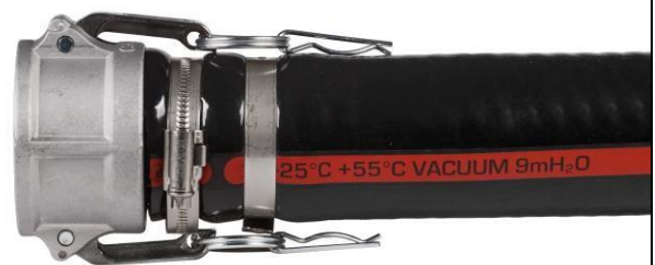
VACUPRESS OIL hose DN50 with CAMLOCK 2" coupling (AC-C-200-AX) in aluminium, assembled with two worm drive clamps (AB-03017543) made of AISI 316 stainless steel.
